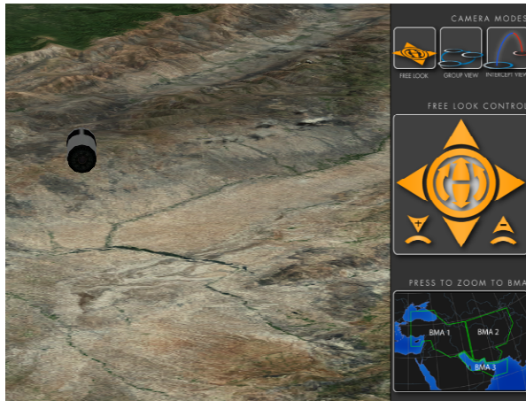
Figure 7. Close-up view of the ScreenPlay control GUI, showing controls to switch between ScreenPlay view modes, control the Free Look view, and zoom to a selected Battle Management Area.
