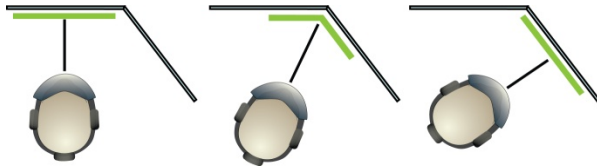
Figure 2. Symbology Bend and Slant Provided by Manipulating Imagery Electronically on the HMD
