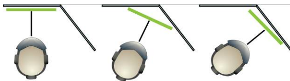
Figure 1. Simplified Overhead View Showing the Geometry Difference Between the HMD Image Plane and Two Adjoining Screens of a Faceted Display System.
