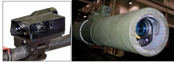
Figure 3 Small arms laser transmitter (SAT) and laser transmitter in gun tube
