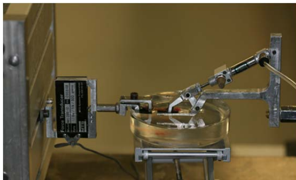
Figure 2. Uniaxial Tissue Testing Apparatus
