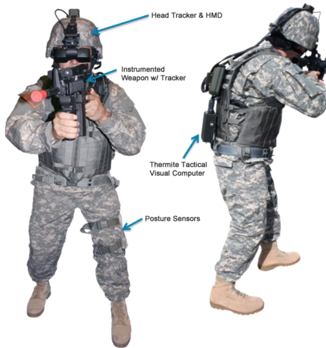
Figure 2. The ExpeditionDI wearable simulation system.
