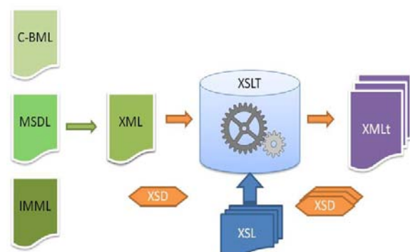
Figure 4. CSES Data Exchange Mechanism logical architecture
