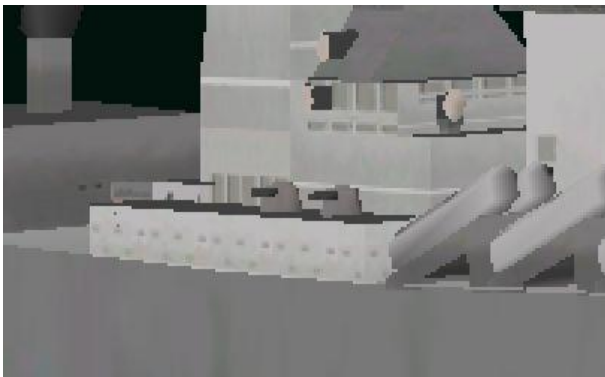
Figure 2 Aliasing Is Inevitable in a Sampled-Data System
