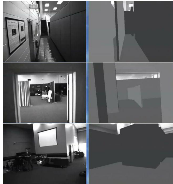
Figure 13. The views rendered from the model using the real-time camera pose estimates by our system for various locations throughout the exercise, together with the real scene views captured by the camera.
