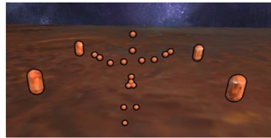
Figure 1: Example of Fusion System in the Unity scene. Each capsule represents a Kinect camera in the lab and the spheres represent skeleton joints.
