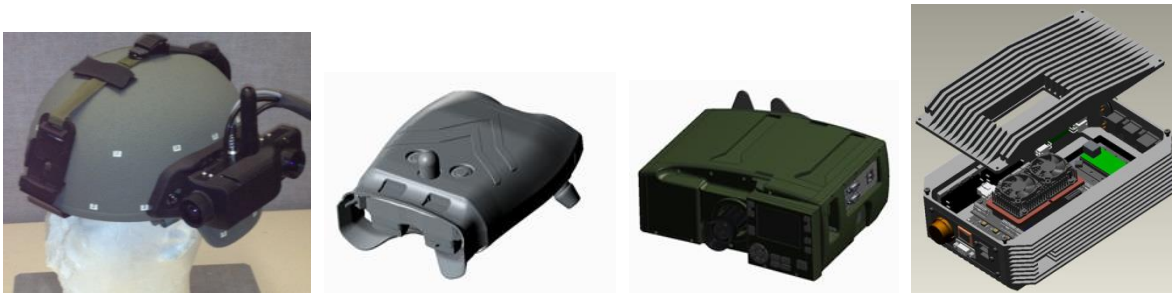
Figure 2. (a) Unaided Eye Sensor Head, (b) Binoculars (c) PLDR (d) Compact Processor.
