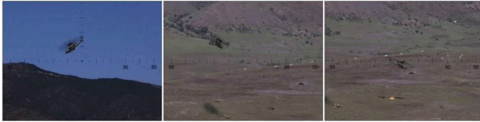
Figure 9. Augmented reality insertion example for AR binoculars. Scene is augmented with helicopter attacking tanks. Tanks and helicopters cast shadows.
