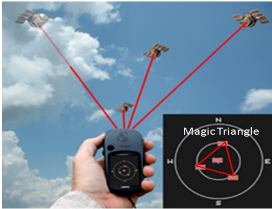
Figure 4. Good GDOP (or HDOP) Geometry
