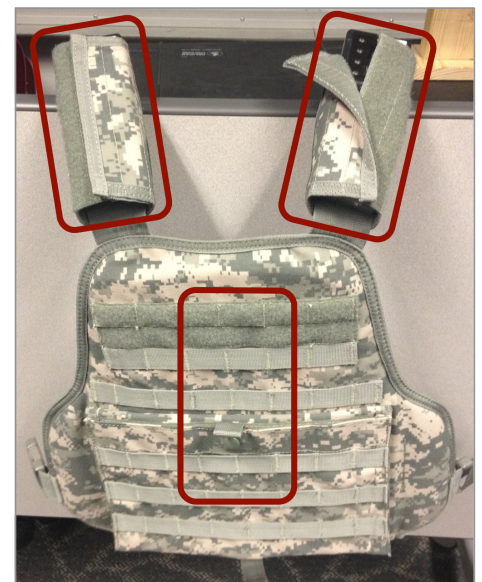
Figure 1: Commercial off-the-shelf pagers were embedded within the vest, two per indicated region.
