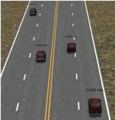
Figure 4 : Several vehicles traveling within lanes. The third vehicle from the left still altered his path some towards the dotted lines to avoid the vehicle in the opposite lane.
