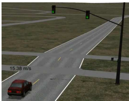
Figure 7 : A green light (represented by Dragons Teeth internally) and a vehicle moving through the intersection (speed displayed above vehicle).
