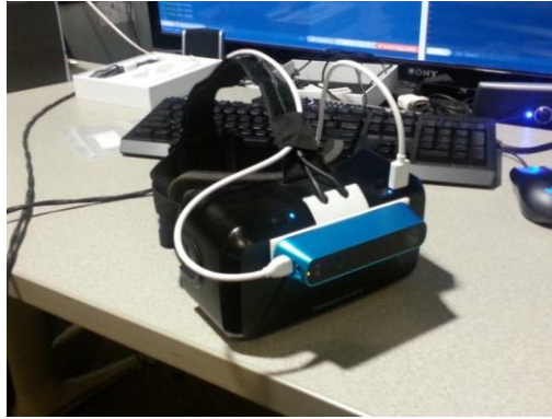
Figure 2. An Oculus Rift with a Structure Sensor (blue) attached to the front.
