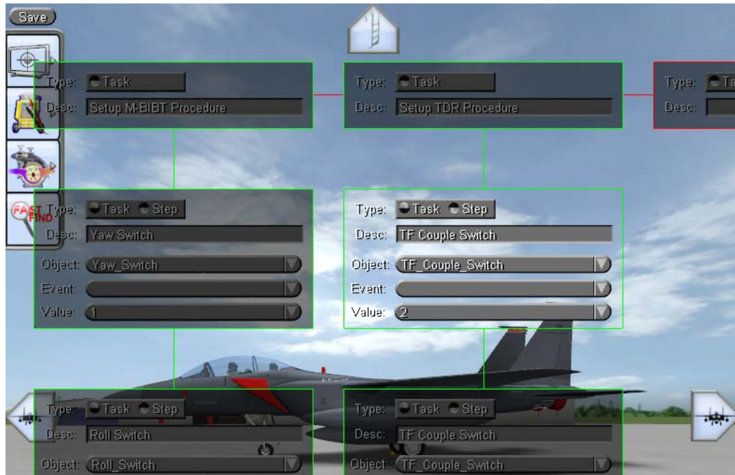
Figure 2: Authoring tool for constructing maintenance training procedures by performing tasks within the game-based simulation
