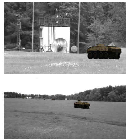
Figure 13. Augmented views from the RWS on the surrogate test vehicle
