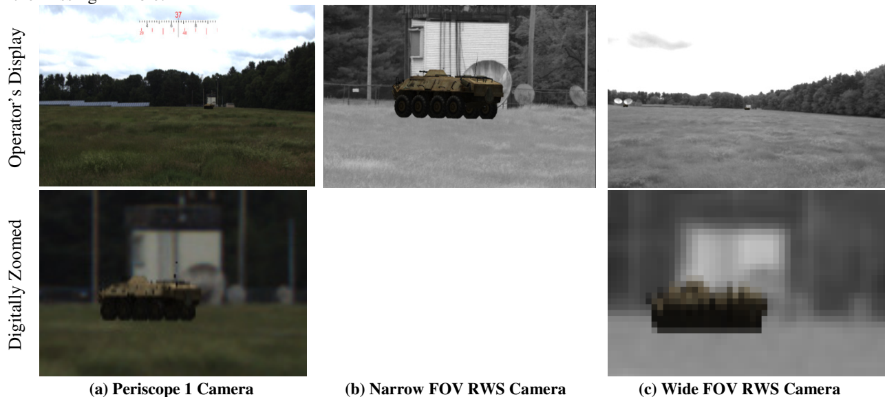
Figure 14. The top row shows the operator's view of the same AR target from three different cameras. The bottom row shows digitally zoomed views of the (a) and (c) cameras for comparison with (b). The difference between (a) and (b) is due to the physical camera offset for a 250m target.
