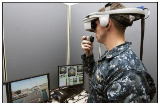
Figure 5: COVE student with VR HMD and voice command microphone. The right monitor shows engine/rudder/speed status; the left monitor is a repeat of the student's FOV (Photo credit U.S. Navy)
