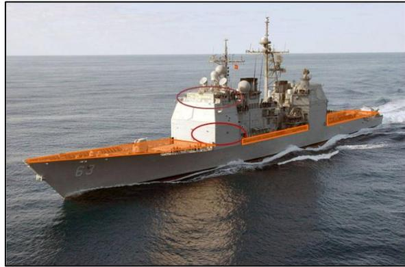
Figure 1: Guided Missile Cruiser USS COWPENS with bridge, CIC, and deck C2 nodes highlighted (photo credit U.S. Navy)
