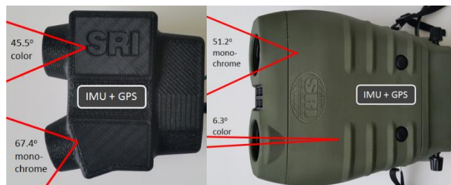
Figure 6. Helmet attached unaided eye and hand-held binoculars each include a wide FoV monochrome camera for robust tracking and narrow FoV color camera for augmentation and precision tracking.
