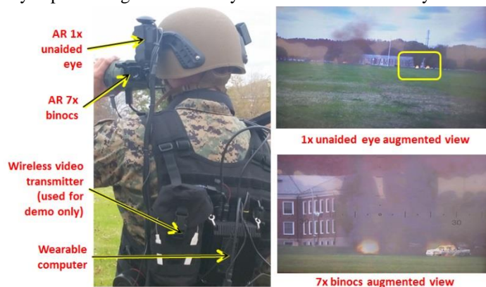
Figure 1. The two-in-one system displays the real world augmented with virtual elements such as targets and explosions. Unaided eye and magnified binocular views are shown on the right.
