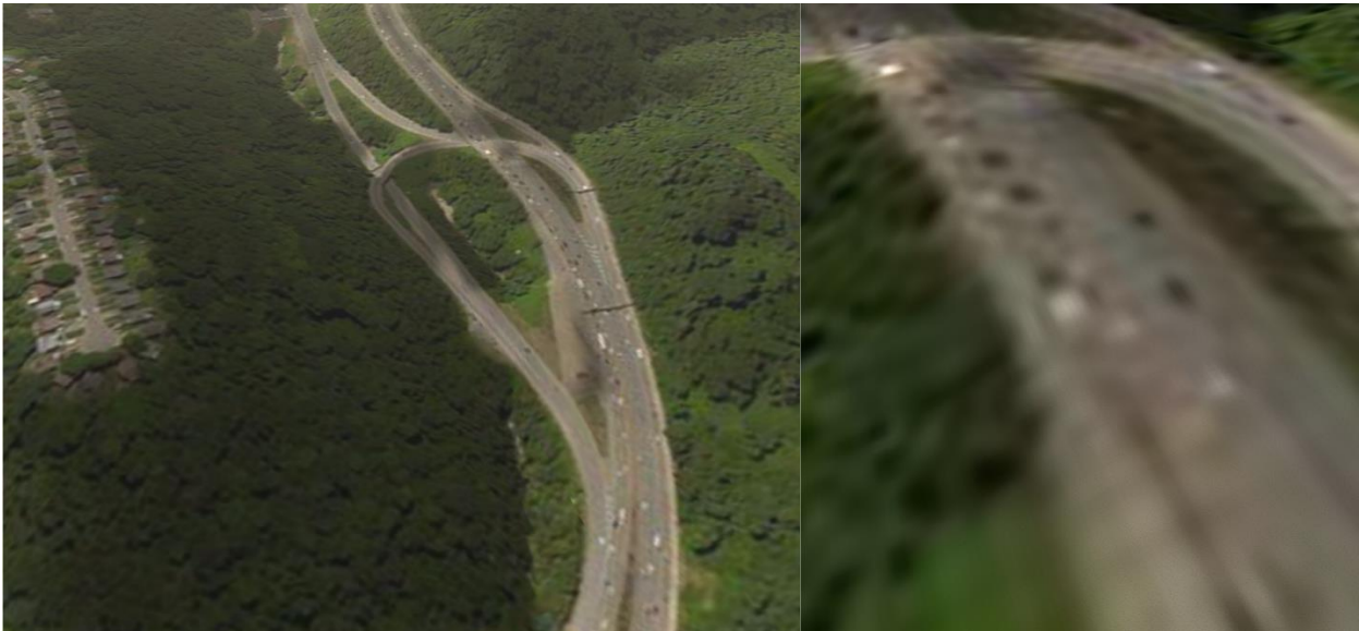
Figure 1. The image on the left shows how vehicles can appear on roads when using photo imagery as the ground texturing, which may create training confusion in MS&T systems. The image on the right demonstrates the blurriness of the photo imagery when visualizing close to the ground, making situational awareness within the MS&T system difficult.
