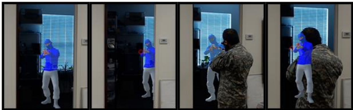
Figure 1. Examples of Occlusion. Leftmost is a hologram of an OPFOR. Next the hologram is statically occluded by the wall. Right of that is a scene that demonstrates proper dynamic occlusion. The final scene is what happens when there is no dynamic occlusion.
