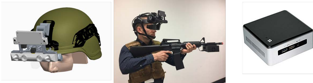
Figure 8. Sensor Head with HMD on NVG Mount, Full AR System with AR-weapon, Intel NUC Processor.
