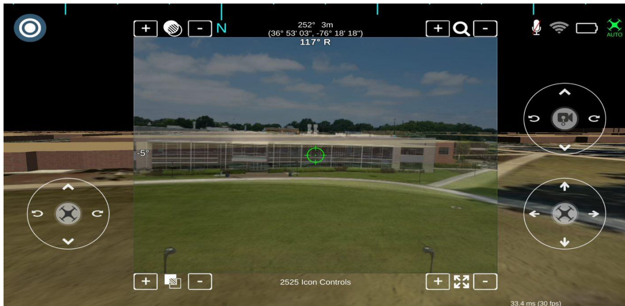
Figure 1. FAR/SV presentation as viewed by an SUAV operator with live sensor feed in the center of the FAR/SV display with blue sky conformally fused with synthetic imagery with black sky showing the surrounding terrain and cultural features such as roads and buildings. The difference between the real-world blue sky and the synthetic vision is purposeful towards enabling intuitive visualization of the different contexts. FAR/SV provides a wider field of view visual context to the operator enhancing situation awareness while maintaining high sensor resolution for the principal area of interest.
